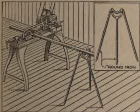
Stock Support for Power Hacksaw: The Height of the Tripod can be Varied by Changing the Spread of the Three Legs
